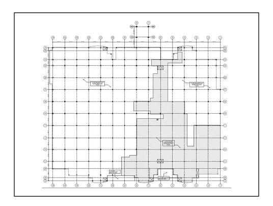
Note how the building exterior (re-entrant corners) drives the location of some grids. This is how the building exterior drives the grid spacing.
