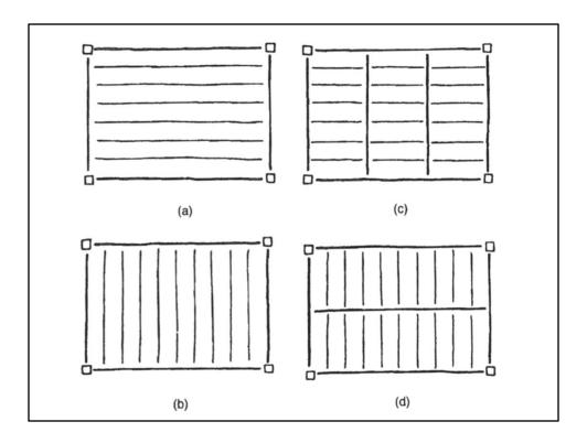
The bay size is controlled by the column layout. Here a rectangular bay allows for multiple framing scenarios. Because of span limits one might choose these framing systems and materials:
