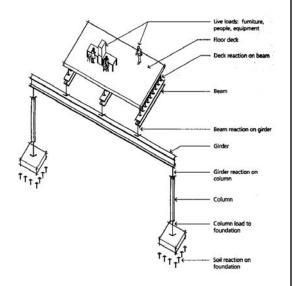
The *load path* is the route that loads take from their source to their final destination (the ground). In conventional framing systems, the load travels from its source to the *deck*, then to *joists* or *beams*, then *girders*, then *columns*, then the *foundation*, which bears on soil.
